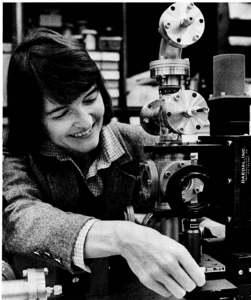
CAROL ASHBY (1126) adjusts the mounting fixture that holds samples of semiconductor materials ready for etching by a laser beam. Carol has used tunable dye lasers to achieve the right wavelengths for etching specific materials.
